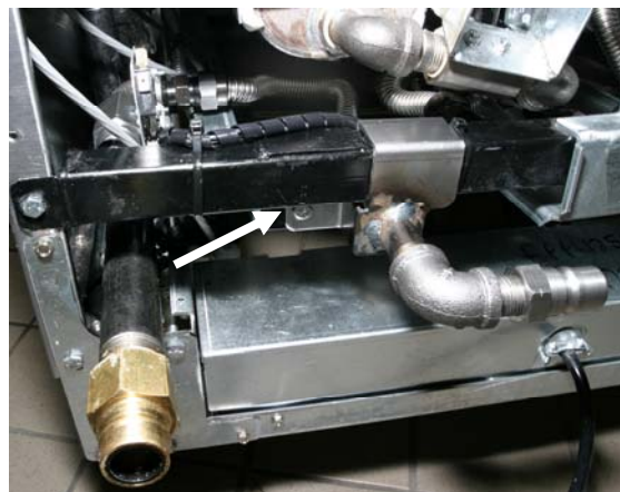
Figure 3*: The assembly is shown in place. The quick disconnect is secured with the existing mounting bolt on the rear return manifold (see arrow).
