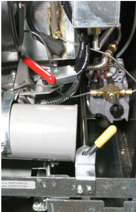
Figure 6: The oil discharge lever bracket attaches to the cross piece in the front of the fryer.
