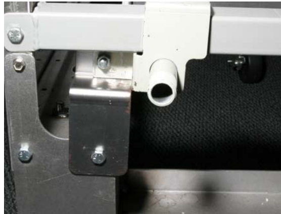
Figure 7: The rear-discharge plumbing is mounted as shown above on three and four-vat fryers.
