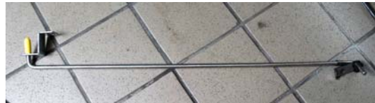
Figure 5 The oil-return activation rod is shown with its hardware attached.
